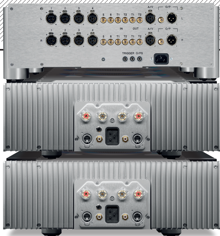
ABOVE: Preamp [top] offers eight line ins (four on XLRs, four on RCAs including two tape loops), one AV bypass output (on XLRs) and two sets of main outputs (on RCAs and XLRs). The power amps [below] have inverting and non-inverting inputs on RCAs and balanced XLRs with partnering sets of speaker outputs on 4mm binding posts
